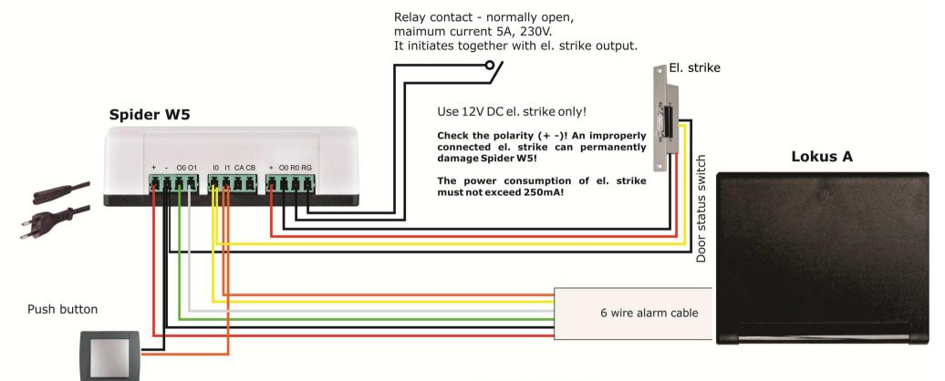
Connect the Lokus to the Spider W5 power supply as shown in the diagram with a standard UTP cable.
