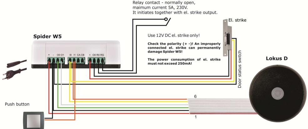
Connect the Lokus to the Spider W5 power supply as shown in the diagram with a standard UTP cable.
