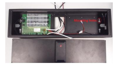
3. Pull the cables through the back hole in to the NEO K unit.
