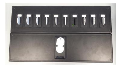
You can see, that this key-tag needs to be in slot nb.7 since the green LED is lit after the key-tag registration.
