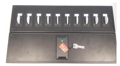
2. Remove the key-tag from the slot by hand.
