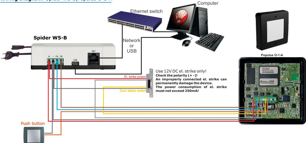
Connect Populus to the Spider W5-B power supply as shown in the diagram with a standard UTP cable.
