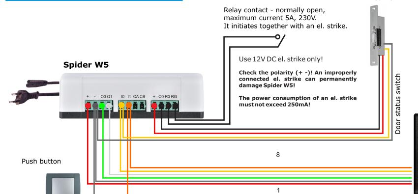
Connect the controller to the Spider W5 power supply as shown in the diagram with a standard UTP cable.
