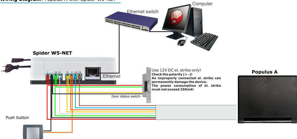
Connect controller to the Spider W5-NET power supply as shown in the diagram with a standard UTP cable.
