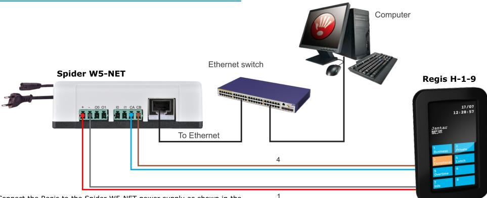
Connect the Regis to the Spider W5-NET power supply as shown in the diagram with a standard UTP cable.
