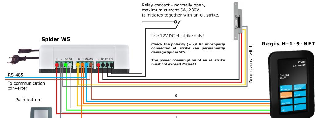
Connect the Regis to the Spider W5 power supply as shown in the diagram with a standard UTP cable.
