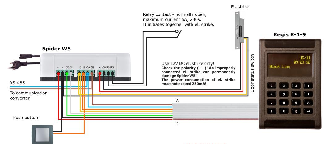
Connect Regis to the Spider W5 power supply as shown in the diagram with a standard UTP cable.
