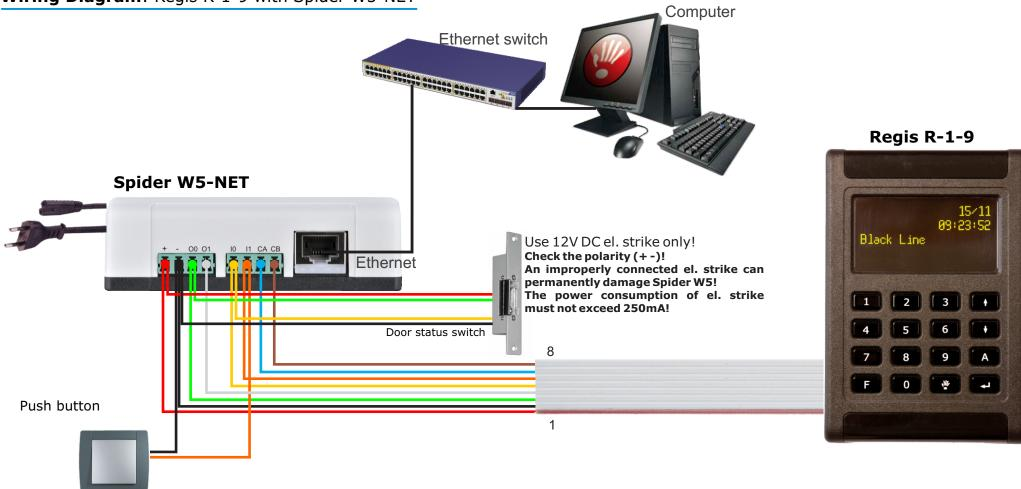
Connect Regis to the Spider W5-NET power supply as shown in the diagram with a standard UTP cable.
