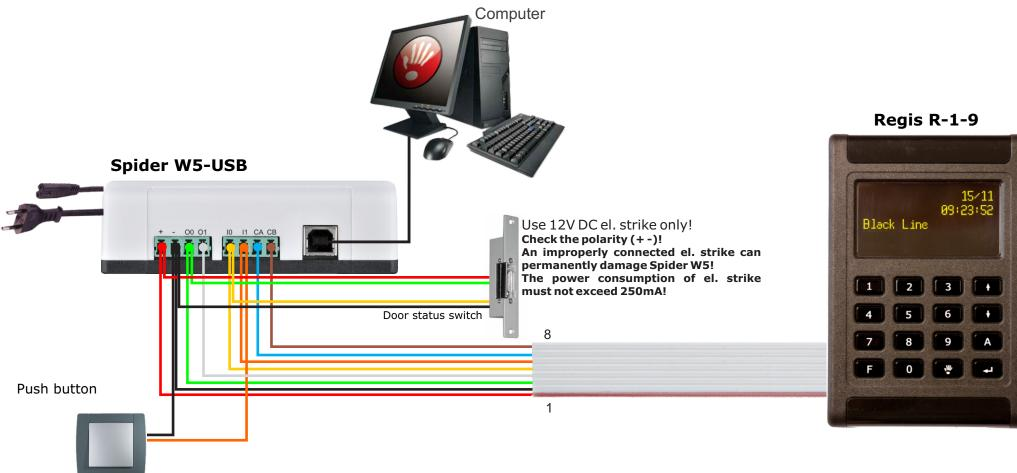
Connect Regis to the Spider W5-USB power supply as shown in the diagram with a standard UTP cable.
