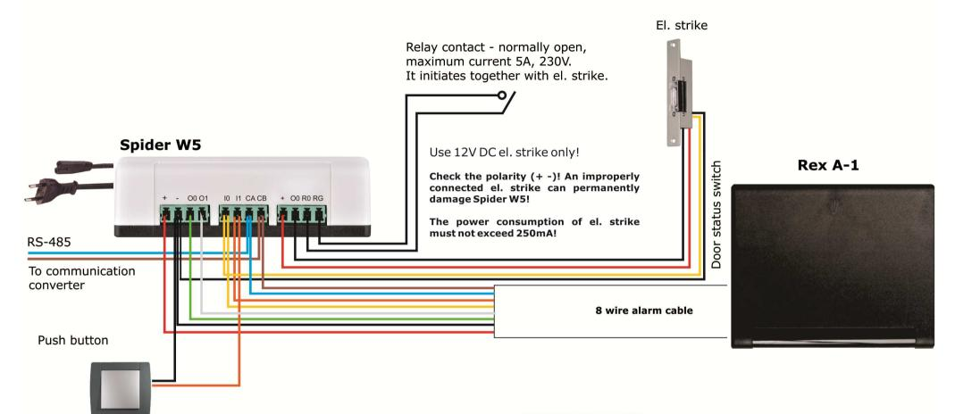
Connect Rex to the Spider W5 power supply as shown in the diagram with a standard UTP cable.
