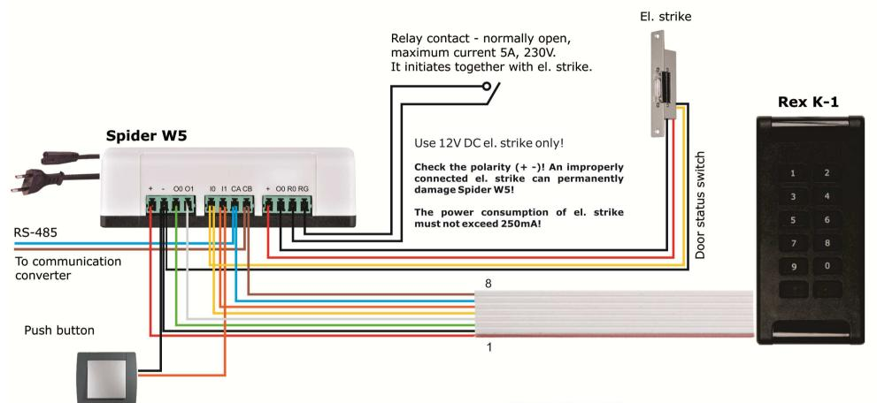
Connect Rex to the Spider W5 power supply as shown in the diagram with a standard UTP cable.
