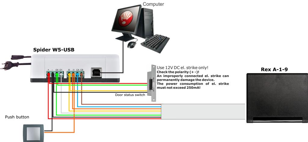
Connect Rex to the Spider W5-USB power supply as shown in the diagram with a standard UTP cable.
