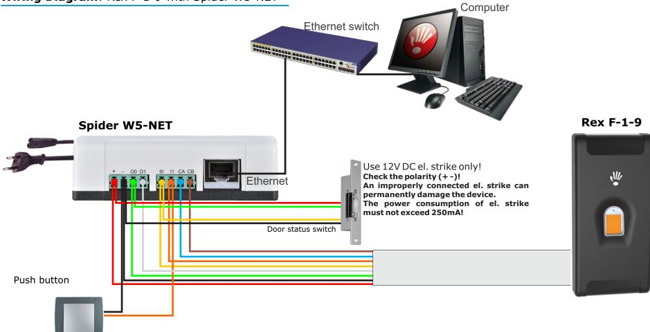
Connect Rex to the Spider W5-NET power supply as shown in the diagram with a standard UTP cable.
