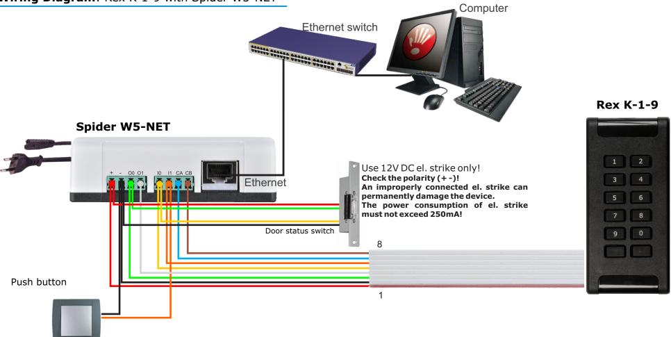
Connect Rex to the Spider W5-NET power supply as shown in the diagram with a standard UTP cable.
