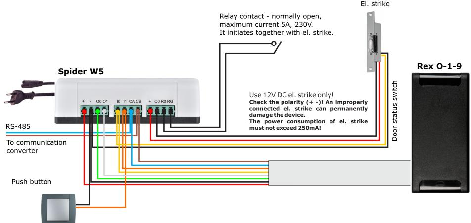
Connect Rex to the Spider W5 power supply as shown in the diagram with a standard UTP cable.
