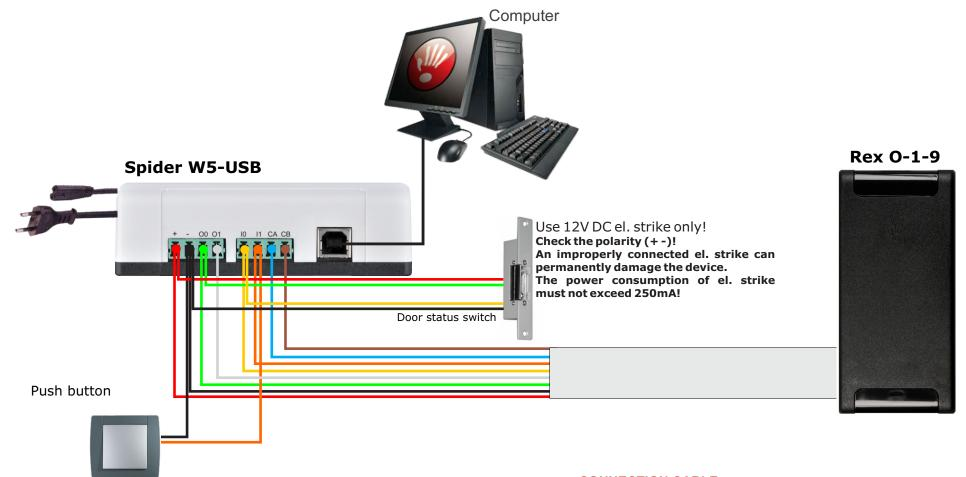
Connect Rex to the Spider W5-USB power supply as shown in the diagram with a standard UTP cable.
