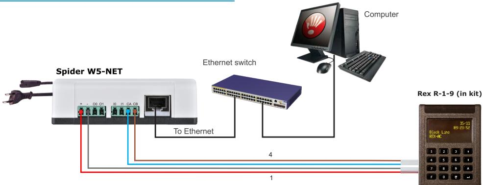
Connect the Rex to the Spider W5-NET power supply as shown in the diagram with a standard UTP cable.
