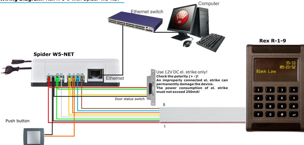
Connect Rex to the Spider W5-NET power supply as shown in the diagram with a standard UTP cable.
